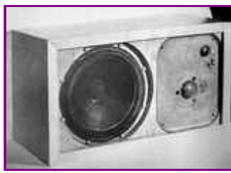
"Prototype of AR-3 speaker system, including AR-1 acoustic suspension woofer and the two tweeters described in this article," from Audio , Oct. 1958
